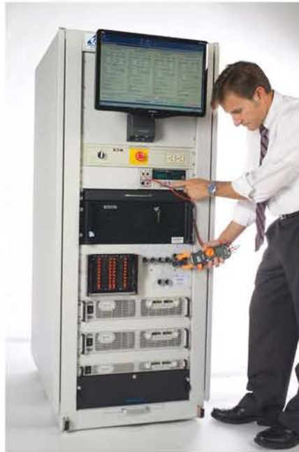
Cable Access in Front for Clip-On Meter
