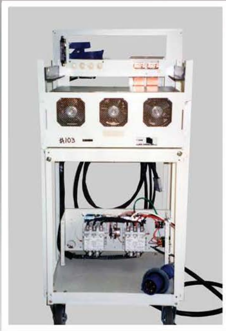
Burn-In Cart with lower cover removed showing contactors
