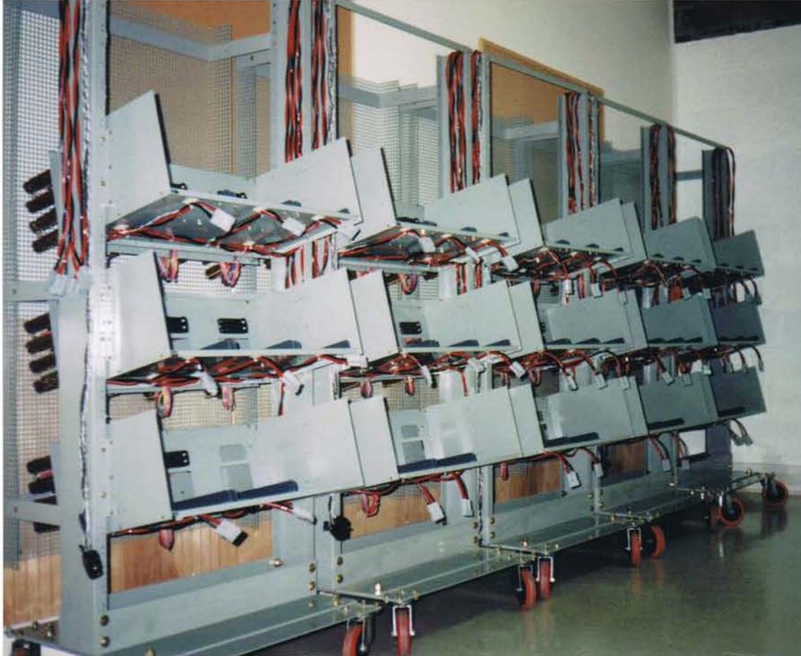
Front view of Multiple Burn-In Carts
