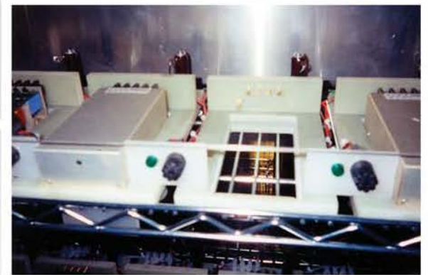
LED and Fuse for each Slot
