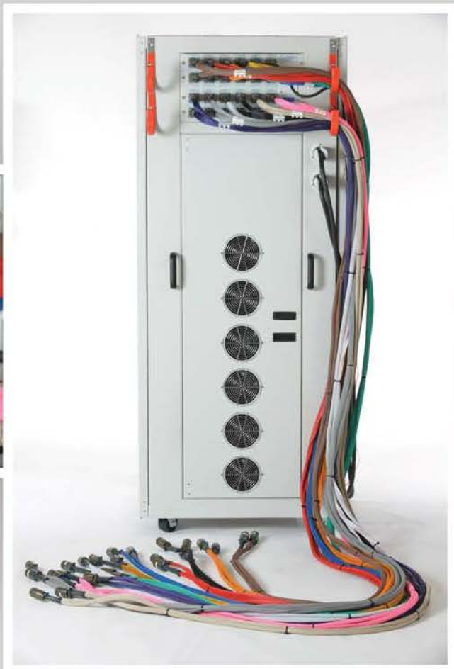
Rear View showing 12 Thermally Rated and Color Coded UUT Test Cables from Chamber to System
