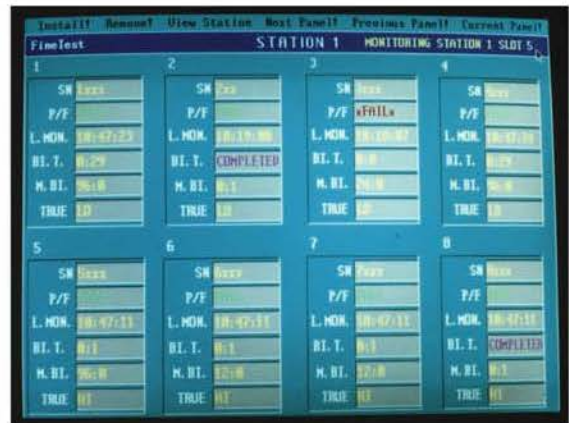
FineTest Burn-In Monitoring Software
