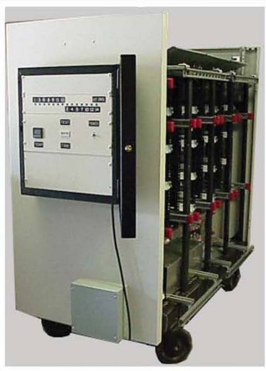
Side view of Life Test Burn-In Cart showing AC Input Power Control Box with Power Cycling Timer
