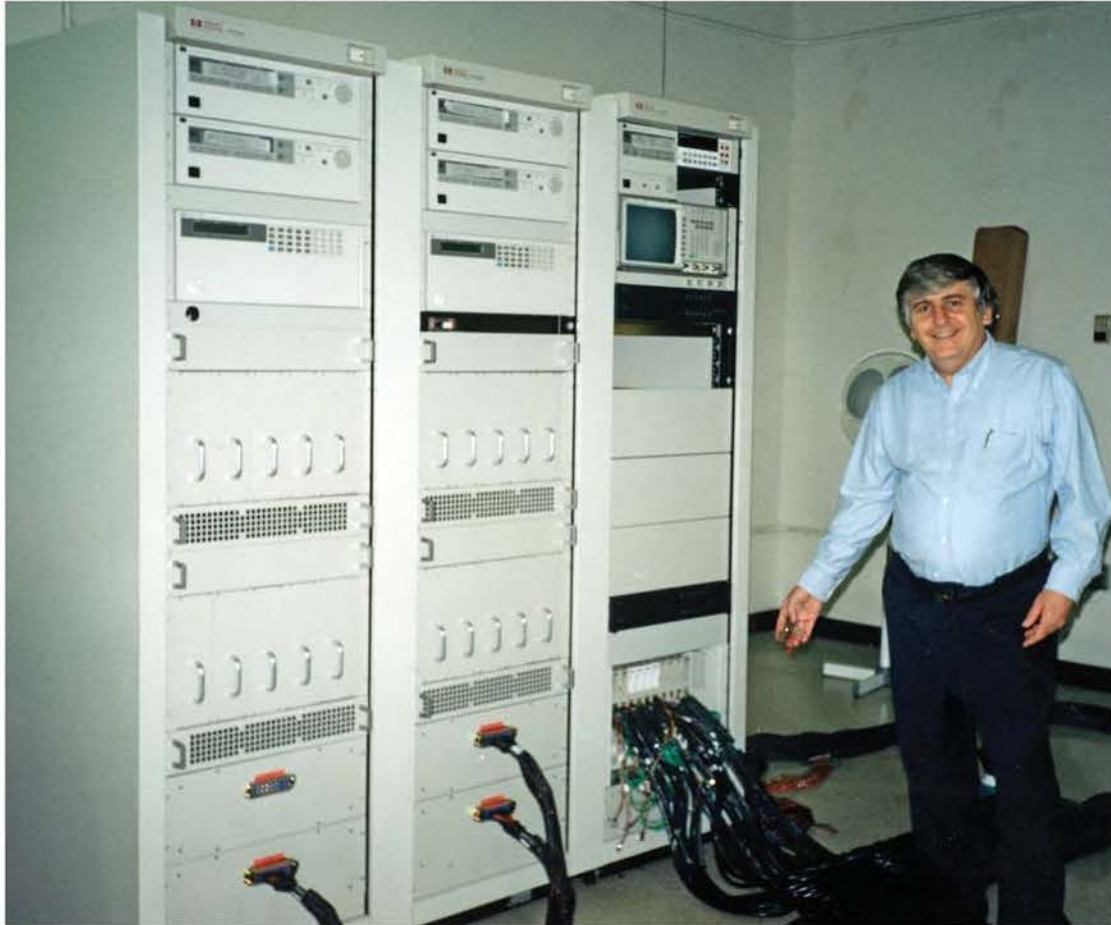
Front view of Tester showing 20 Burn-In Loads, Power Switching Units, VXI Switching
