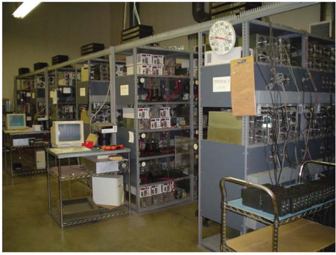
Close-Up of Multiple Burn-In Systems
