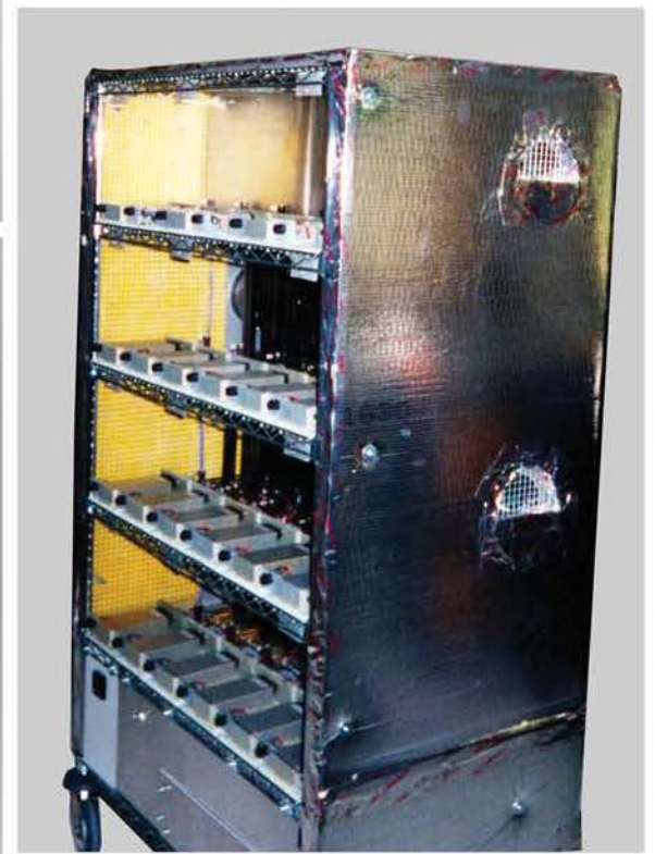
Heat Exhaust Fans on Side of Cart
