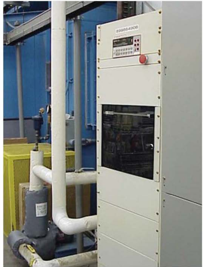
Front view of Burn-In Monitoring System Integrated with Thermal Chamber
