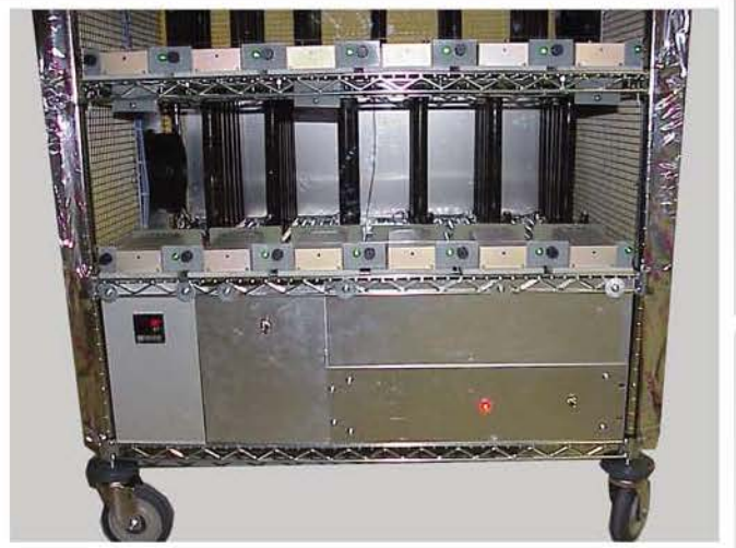
Close-Up of Temperature Controller and Power Control Box
