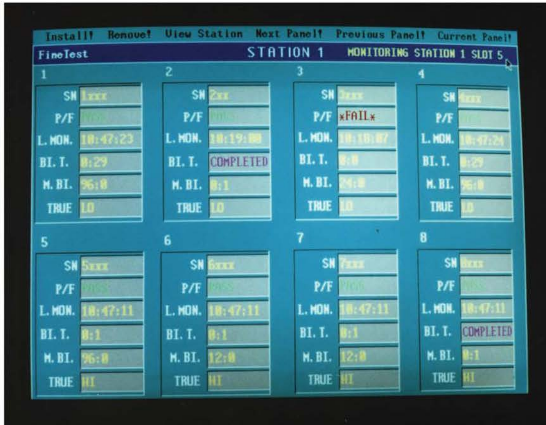
Front view of FineTest Burn-In Monitoring Software
