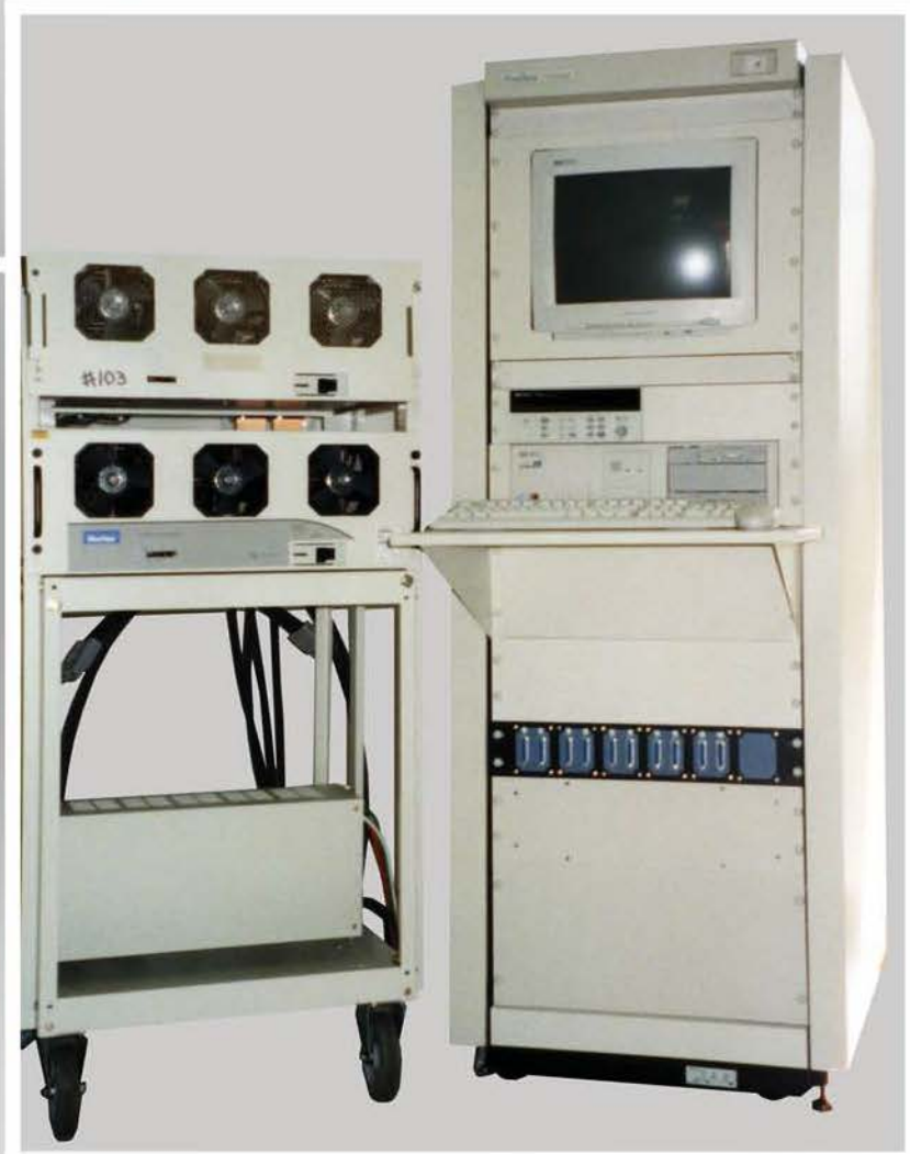
Burn-In Monitoring System and Cart with 2 UUTs
